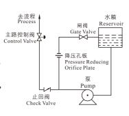
The bypass is constant operate and recirculate flow through orifice plate to reservoir, It's effective. However this continuous recirculation would require oversized pump and leads to extra energy consumption.
