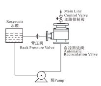
Automatic recirculation valve combine the check valve, flow meter, bypass control valve, multistage letdown function into one integration unit. No power or signal source needed, static seal design, zero leakage, zero electricity, intrinsic safety, minimized the connection point, saved installation and maintenance cost.
